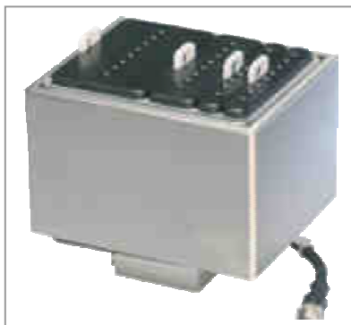
Figure 1: Peltier elements facilitate reagent or sample temperature control. The example shown is a modular reagent trough rack – the troughs are removable and the many possible trough combinations are user-configurable.
